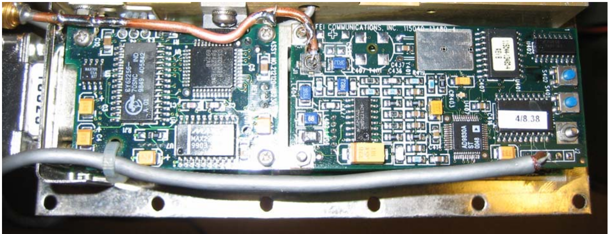
Detailed view of the DDS board where the 2 cables are connected to the PCB
