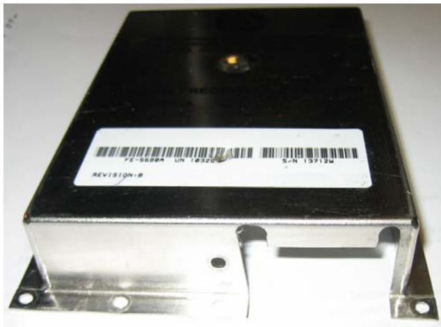
Modified lid to route the RF and RS232 signals out
