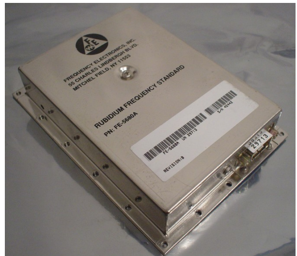
Rubidium Frequency Standard FE-5680A
