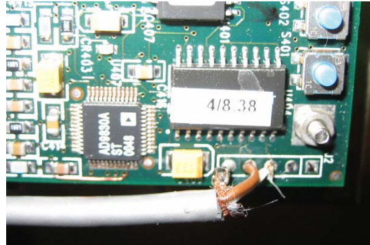
Detailed view of the RS-232 connection
